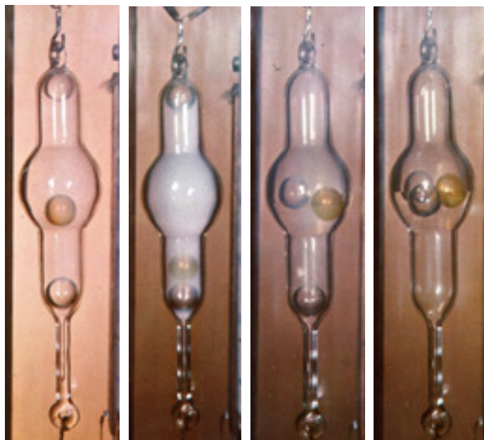
Figure 8.2.6. Glass bulb filled with \text{CO}_2 at a value of V/n close to the critical value, viewed at four different temperatures. The three balls have densities less than, approximately equal to, and greater than the critical density. 8.2.6
